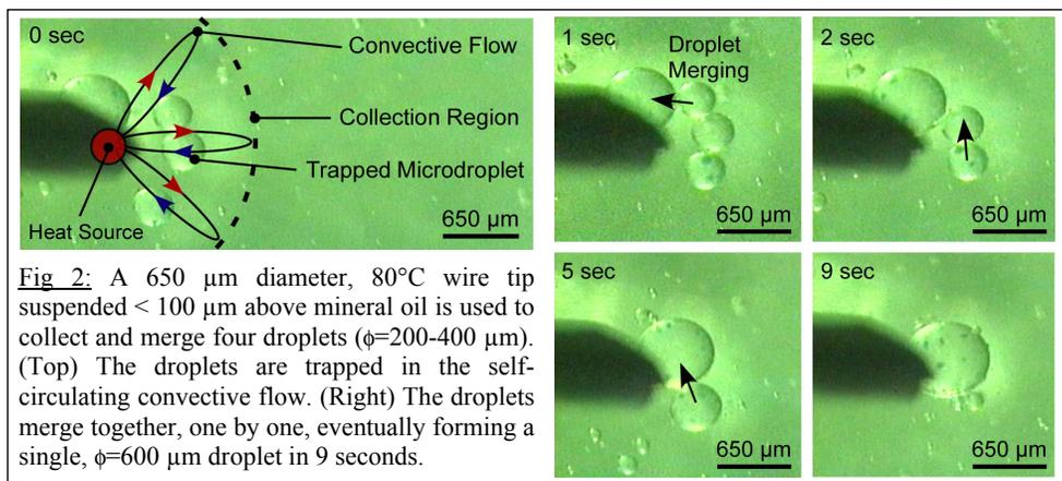
**Fig 2:** A 650  $\mu\text{m}$  diameter, 80°C wire tip suspended  $< 100 \mu\text{m}$  above mineral oil is used to collect and merge four droplets ( $\phi=200\text{-}400 \mu\text{m}$ ). (Top) The droplets are trapped in the self-circulating convective flow. (Right) The droplets merge together, one by one, eventually forming a single,  $\phi=600 \mu\text{m}$  droplet in 9 seconds.
