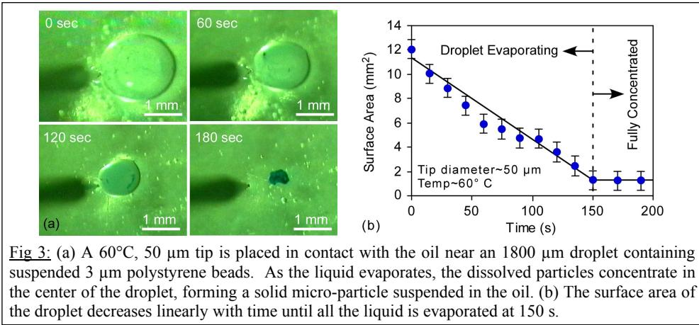
**Fig 3:** (a) A 60°C, 50  $\mu\text{m}$  tip is placed in contact with the oil near an 1800  $\mu\text{m}$  droplet containing suspended 3  $\mu\text{m}$  polystyrene beads. As the liquid evaporates, the dissolved particles concentrate in the center of the droplet, forming a solid micro-particle suspended in the oil. (b) The surface area of the droplet decreases linearly with time until all the liquid is evaporated at 150 s.
